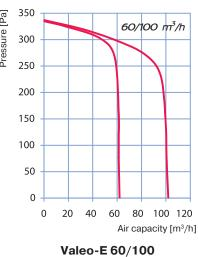
The abrupt curves show high pressure performance and constant air flow of several Valeo-E fans integrated into a single ventilation shaft.
